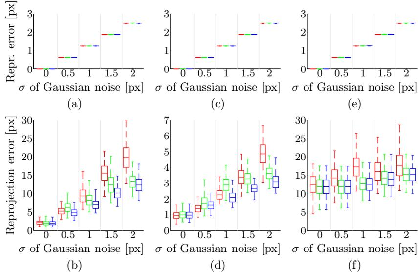
Fig. 2: *Image noise experiment.* Methods BA, SO, and ASO in red, green, and blue, respectively, on calibration and validation data point sets. (a–b) barrel distortion, (c–d) pincushion distortion (e–f) zero-crossing problem.
