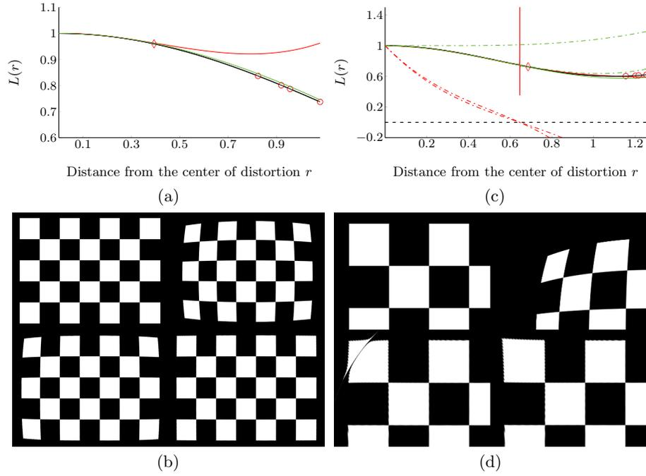
Fig. 1: *Calibration issues.* Examples of issues arising while using polynomial and rational function for radial distortion calibration. See text for details.
